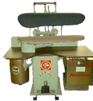
Self Contained pressing unit completely pre-piped ready for on-site connections.
