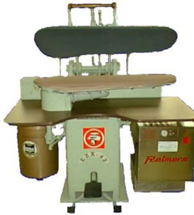
Self Contained Mini Package shown with a 42" manual utility press
